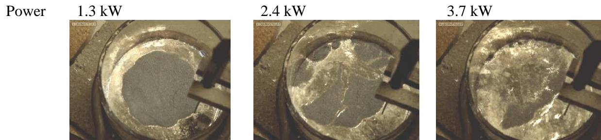
Fig. 3. The surface of the Wood's metal with iron particles after 10 s of steering in the small experimental ICF-1 (6 kg). The particles were situated on the surface before steering (like on the left picture).
