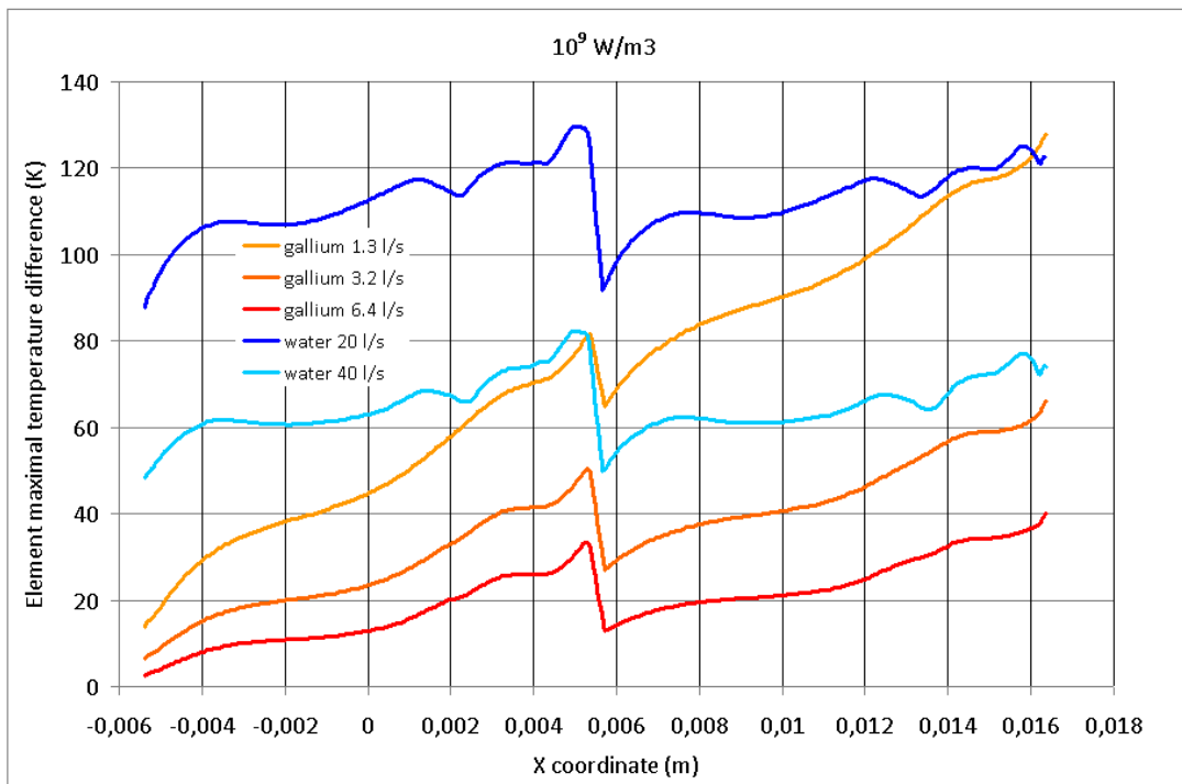
Fig.7. Temperature difference distribution on the rod surface for water and gallium cooling.
