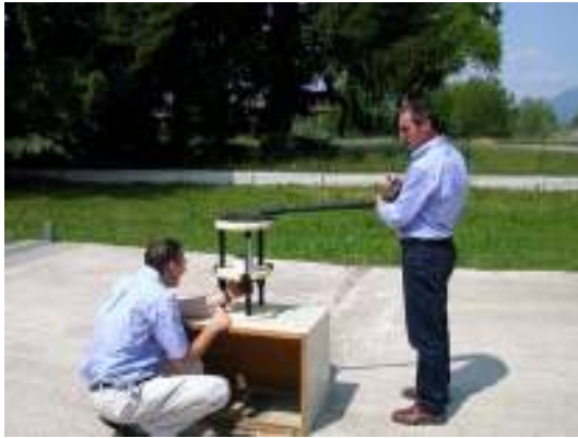
Fig. 3-4 Use of manual jig to determine detector sensitivity.
