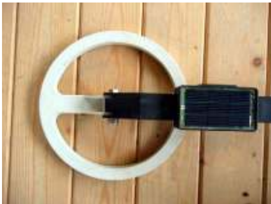
The solar panel (right) is mounted on the search head shaft
