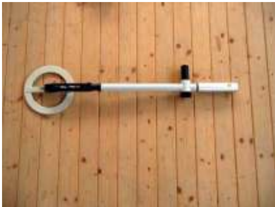
The detector in short configuration with the rechargeable battery pack The armrest and handle are not displayed
