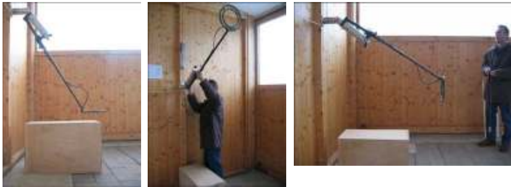
Fig. 10-1 Mounting of a detector on the pendulum for measurement of moment of inertia. The detector is first attached to the “forearm” and extended to a standard length and angle – left hand photo. The “elbow” is unlocked and moved through 90°, so that the detector coil is in a vertical plane, and re-locked – centre photo. The forearm pivot is carefully allowed to rotate 180° about the horizontal axis to the equilibrium position – right hand photo. The period of oscillations of the pendulum about this axis is used to determine the moment of inertia about what would be a vertical axis when the detector is in normal use.
