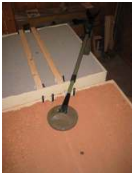
Fig. 3-3 View of the soil boxes from above, with a Minelab F1A4.
