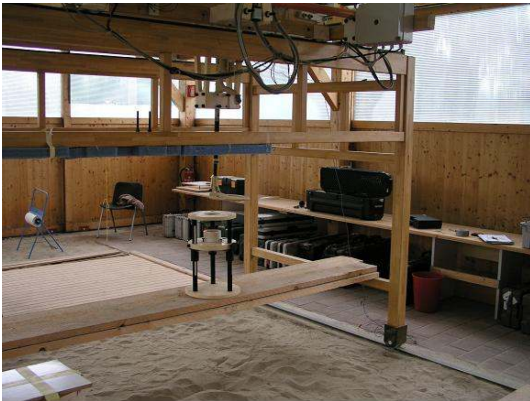
Fig. 3-1 View of Gauss lab main hall, showing positioner with a detector mounted
